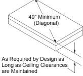
Figure 8 - Appliance Must Be Installed on a Wood or Metal Panel if Being Installed on Any Combustible Material Other Than Wood
